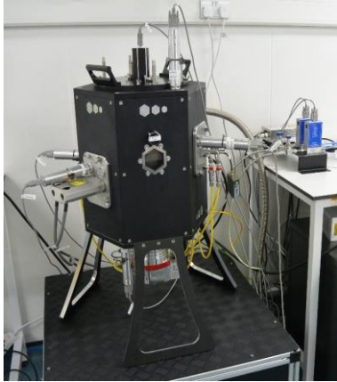
OXIS Lab-scale sputtering System
