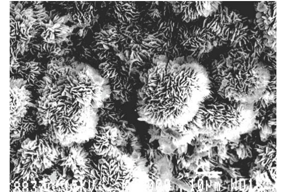
Photo SEM LMDC – SAR gel
