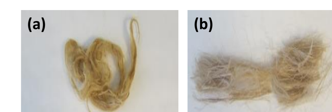
Figure 6. Visual comparison of a) fiber treated with NaOH 5% and b) untreated fibers.
