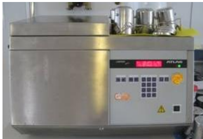
Lini-test washing device : based on ISO 105-C06:2010.
