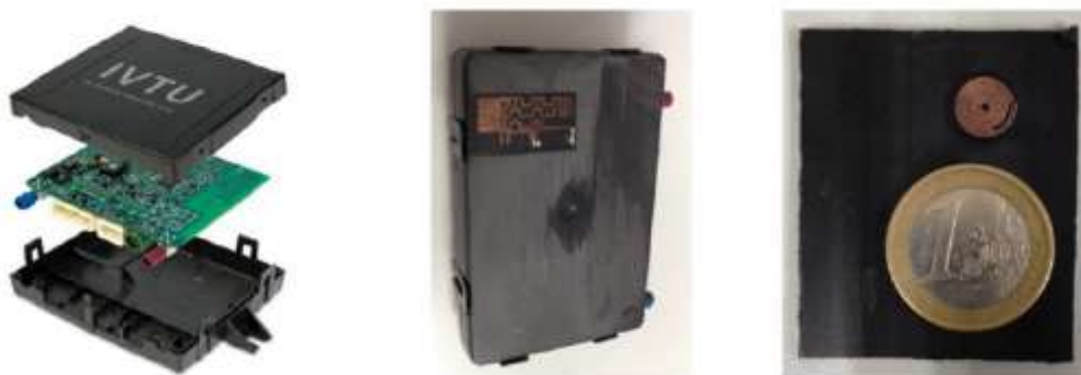
Figure 2: Current FICOSA Telematic Unit, Adapted prototype with a printed antenna, and a printed inductor sample, created by the Orf4Auto Project
