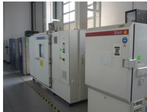
Climatic chamber (without/with light (MHL)) also Xenotest and UV chamber from Atlas
