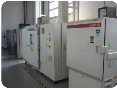
Climatic chamber (without/with light (MHL)) also Xenotest and UV chamber from Atlas
