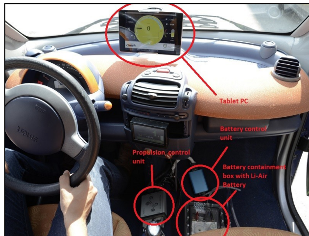
Li-air battery setup in a car
